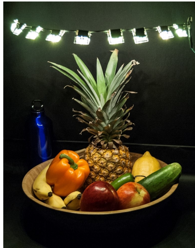
Photo illustrating good color rendering of the SWOLEDs in this report. The luminaire comprises 36 pixels (2 mm 2 ) operated at 50-100k nits
